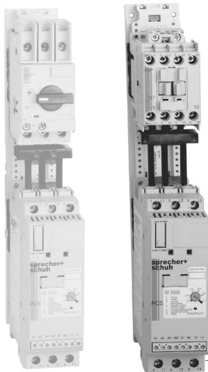
Sprecher + Schuh DIN-rail mounted Controllers can be direct connected to CA7 contactors to provide isolation or to KT7 Motor Circuit Controllers for branch circuit protection (for models up to 37A)
