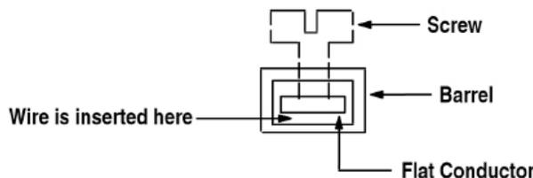
The screw is not threaded into the flat conductor but rather bears against its top surface. This causes the barrel to be drawn upward clamping the wire between the undersurface of the flat conductor and the lower portion of the barrel. A major advantage is the wire is easy to insert into the clamping area.
