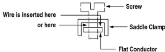
The saddle clamp should be designed so it tilts to securely clamp a single wire on one side or a different wire size on each side of the clamp.
